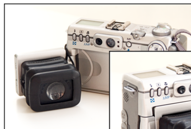
This rubber hood is also attached with Velcro strips.
