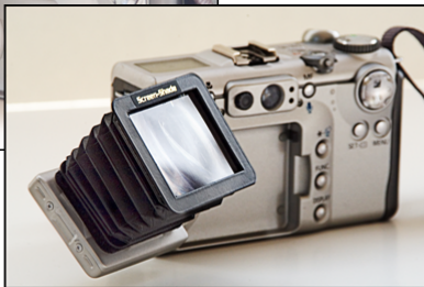
This collapsible hood attached with Velcro strips includes a magnifier.
