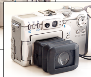
This rubber hood is also attached with Velcro strips.
