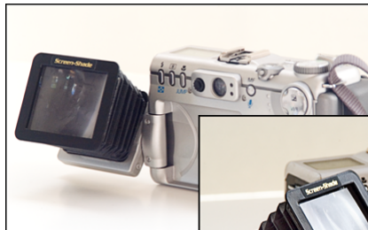
This collapsible hood attached with Velcro strips includes a magnifier.
